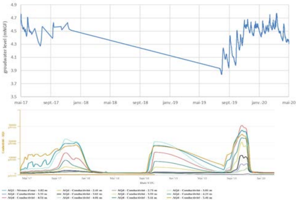
Figure 7: Conductivity and level data acquired by the SMD-AQ4 from May 2017 to July 2020 (up: electric conductivity in \mu\text{S}/\text{cm} at different depths, below: groundwater level in mNGF).
