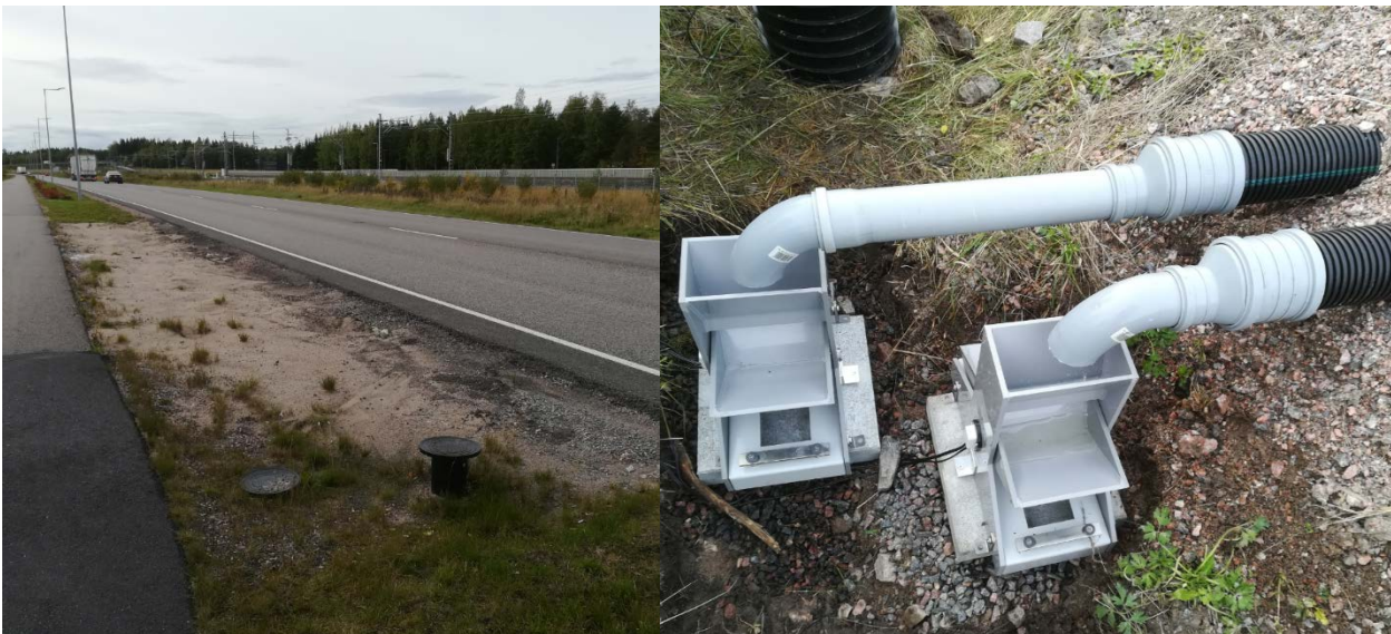
Figure 15: Tikkurilantie roadside filters, and their instrumentation for discharge (tipping buckets).
